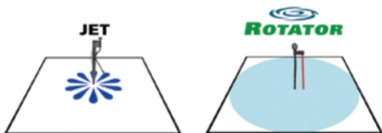
A Rotator sprinkler distributes water uniformly at a rate at which the soil can absorb the moisture.
