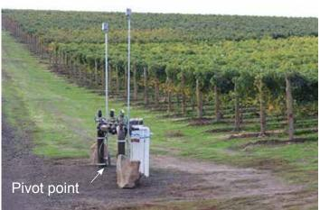
TWIG-2i on a stake in a vineyard. Pivot point to rotate the mast down for access to the TWIG.
