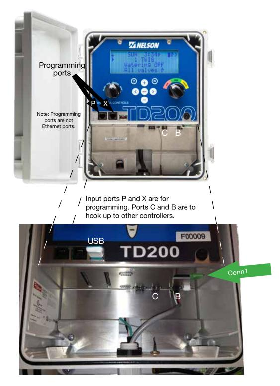
This shows the connection port Conn 1 which is the green port. It can input from a flowmeter or a pause event switch.
