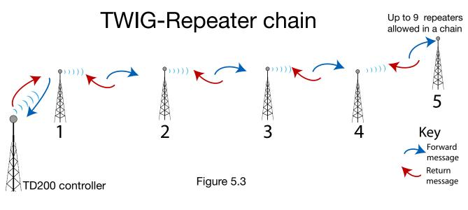
Make sure every link of a Repeater chain is good in order to be reliable! A break anywhere orphans the last end of the chain.
