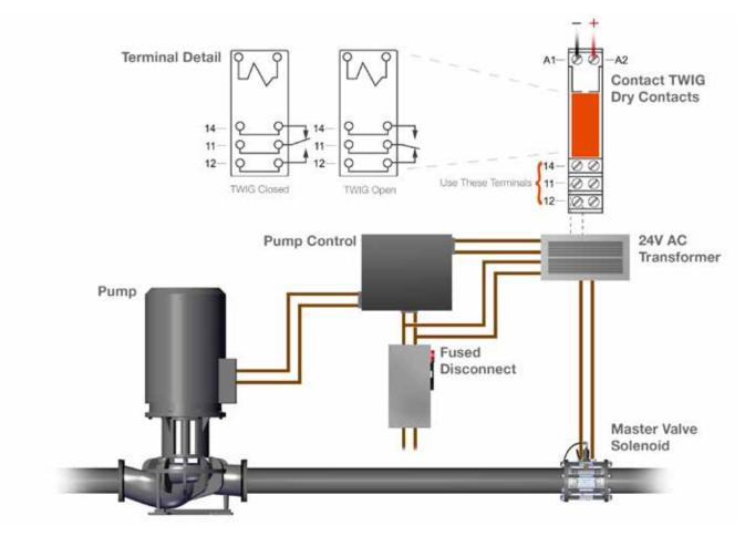
This is a sketch of a typical electric pump layout. In this example one switch is used for the pump and one is used for the master valve. An experienced certified electrician is to make the wiring in conformance with local electrical code).
