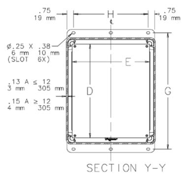
TD200 and Contact-TWIG box dimensions: Mounting hole spacing H=6.56" G=11.38" Contact-TWIG wiring: The four switches in the box are pre-wired from the factory. These switches latch on and off using a momentary 12V DC pulse. The information below is to show the wires into the four switches are color coded because polarity is important to open and close the switches.
