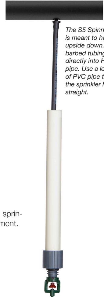
The S5 Spinner is meant to hang upside down. The barbed tubing inserts directly into HDPE pipe. Use a length of PVC pipe to keep the sprinkler hanging straight.
