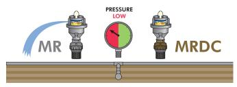
*How they work:* The MRDC and MDC are normally closed devices. The check will not open until a certain minimum inlet pressure is reached. The minimum pressure to open an MRDC is approximately 75% of nominal pressure, and approximately 90% of the nominal pressure for the MDC. Exact regulation with an MRDC will not take place until the inlet pressure is at or above the nominal pressure. Provide 5 PSI above the nominal pressure for the most accurate pressure regulation.
