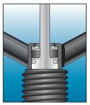
Flow Control Nozzle with low pressure
