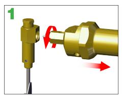
Back-off adjustment screw to remove pressure from the spring. Unthread pilot from stem.
