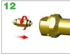
Thread the connector into the reassembled pilot body.
