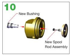
Insert the new bushing (11908) and new spool rod assembly into the spool housing.
