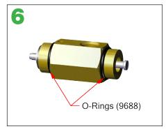
Replace the o-rings (9688) on the threads of the connector.
