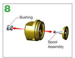
Remove and discard the old spool assembly and old bushing from the spool housing.
