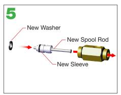
Replace the washer, sleeve (10724), and spool rod (9790) with the parts included in the upgrade kit.
