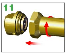
Thread the spool housing back into the spring housing.
