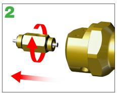
Unthread connector from the spool housing.
