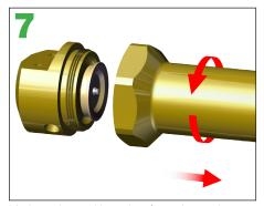
Unthread spool housing from the spring housing.
