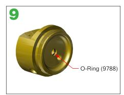
Replace the o-ring (9788) inside of the spool housing. Make sure inside of spool housing is free of debris. NOTE: Use an o-ring pick to remove and replace the o-ring.
