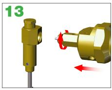
Thread the connector and pilot back onto the stem, making sure the washer is still in place.
