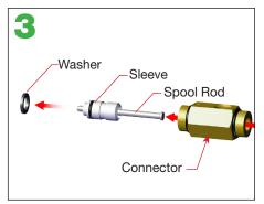
Remove the washer (6495) on the connector. Push the spool rod through the connector to remove both the spool rod and sleeve. Discard the washer, sleeve and spool rod.
