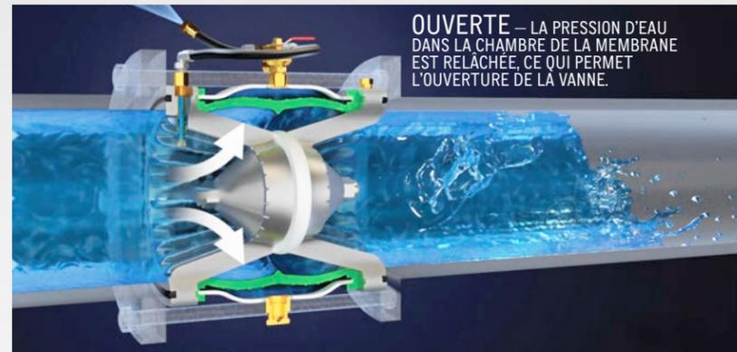
**OUVERTE** – LA PRESSION D'EAU DANS LA CHAMBRE DE LA MEMBRANE EST RELÂCHÉE, CE QUI PERMET L'OUVERTURE DE LA VANNE.
