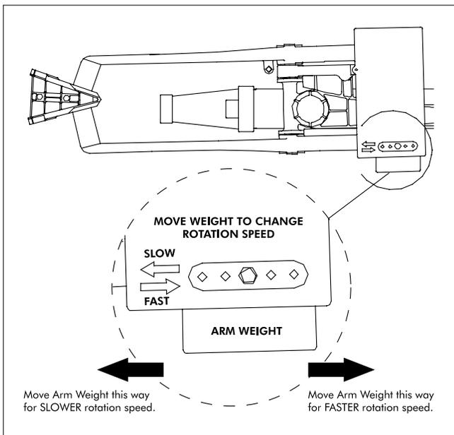
**4.** The SR200 is factory set for normal rotation speed. If a faster or slower speed is desired, move the Arm Weight backward for faster operation or forward for slower operation.
