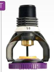
**FLOW CONTROL NOZZLE.** The Flow Control Nozzle (only available for 3000 Series) not only eliminates the need for pressure regulators, but also passes debris more easily. It is not to be used on flexible hose drop assemblies.
