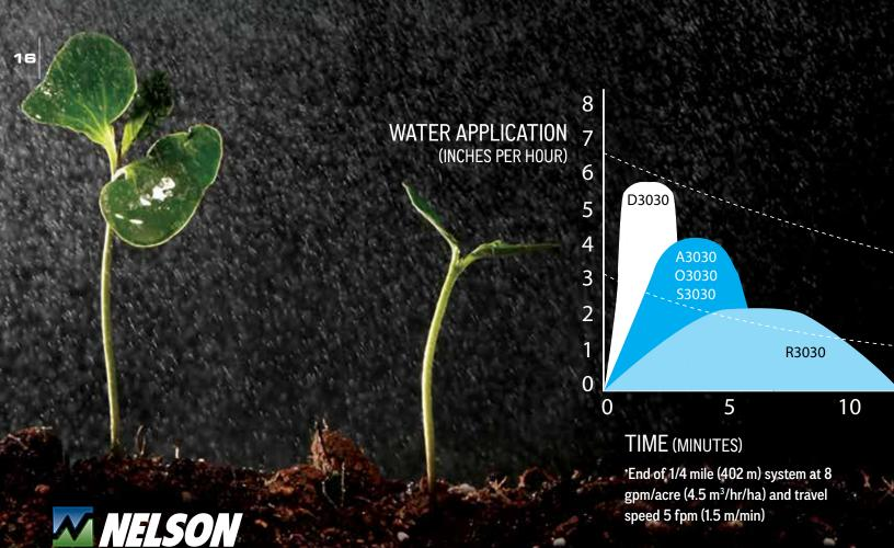
WITH SUPERIMPOSED APPLICATION RATES FOR CENTER PIVOT SPRINKLERS, IT IS OBVIOUS THAT THE ROTATOR®, WHICH PROVIDES THE WIDEST THROW DISTANCE ON DROP TUBES, COMES THE CLOSEST TO MATCHING INFILTRATION RATES OF THE SOIL. THE BEST CONDITION FOR INFILTRATION IS TO KEEP THE SOIL SURFACE OPEN AND APPLY WATER
