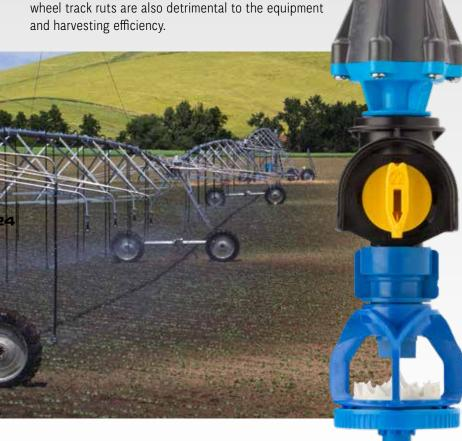
Nelson part circle sprinklers direct the water off of the pivot structure at the towers and away from the wheel track to prevent deep wheel track ruts. Overall field uniformity can be maintained by preventing excessive slippage of the tires, and maintaining a uniform speed of travel.
