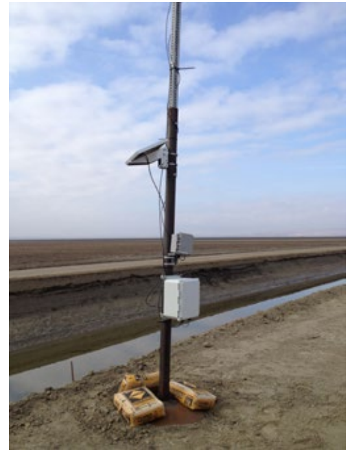
Repeater on a portable stand.
