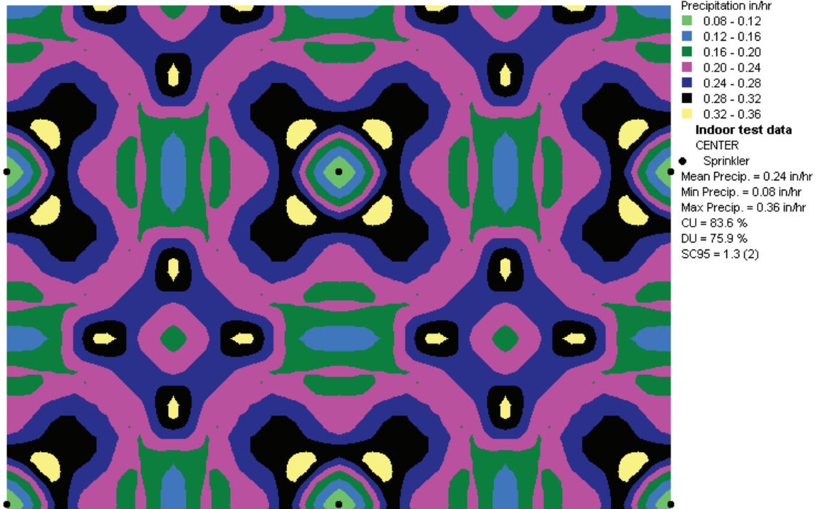
R10TG Black #14 Green 24" 40.00 psi 12.00 in Rec. # R10T test Rect 30.00x30.00 ft Run 2
